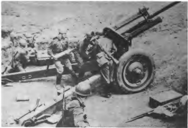
Figure 6-27. 122-mm howitzers. The M-30 (above) and D-30 (below) are the standard divisional artillery weapons in Soviet Ground Forces. The newer D-30 has a maximum range of over 15,000 meters.
